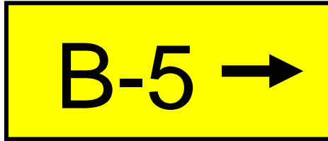
Runway Exit Sign
