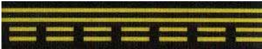
Runway Holding Position Marking
