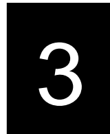
Runway Distance Remaining Signs
